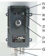
FAIL INDICATOR (red); is lit or blinks when an error is detected.
