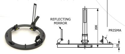
The Azimuth circle measures the fixed error of the gyrocompass. To observe a bearing, the observer looks through the peep vane toward the object to be observed or "shot". The ring is then rotated until the object appears beyond the vertical wire of the opposite "far" vane. The true bearings appear on the compass card above the relative bearings.
