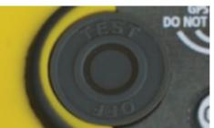
After a few seconds, a good self-test will result in the indicator light flashing a number of times in quick succession depending on battery usage;
