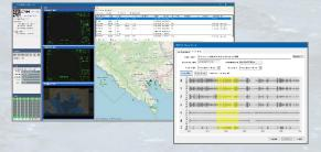
The AMI Marine Replay software is unique due to having '*Audio Scan'* and '*Jump to Incident*' functions to provide intuitive data review by engineers, ship's crew and accident investigators.
